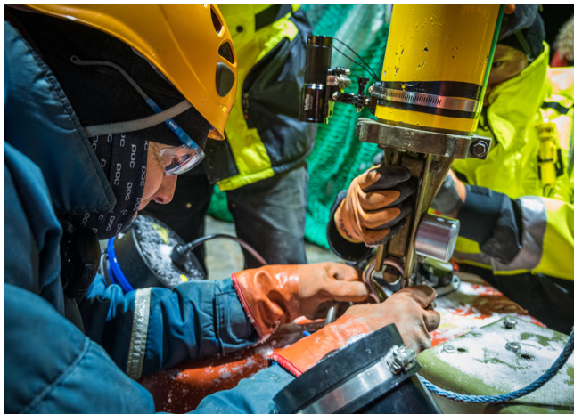
FIG. 3. Dr. Jim Thomson connects an acoustic release to a sea spider tripod, deployed to measure sea conditions at the intersection of waves and ice formation in Beaufort Sea. Photo: John Guillote.
